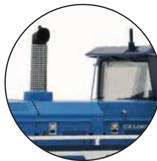
Exhaust pipe panelling made from photo-etched
